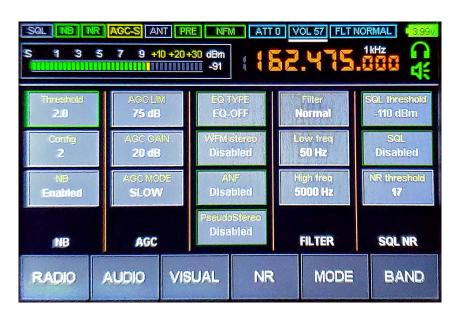
The **AUDIO** menu lets you configure various sound characteristics, such as filtering, gain, noise reduction, noise blanking, and squelch. Touch a menu item to select it. If an item has more than two different values, rotate the larger knob to change between these values. To exit the menu, touch the **AUDIO** button again. This menu contains the following sections.
