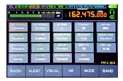
The **RADIO** menu lets you configure various hardware features, such as radio frequency gain, pre-amplifier, attenuator, and so on. Touch a menu item to select it. If an item has more than two different values, rotate the larger knob to change between these values. To exit the menu, touch the **RADIO** button again. This menu contains the following items.
